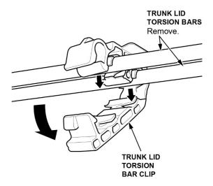
3. Remove the truck lid torsion bars with the torsion bar assembly from both trunk lid hinges.
