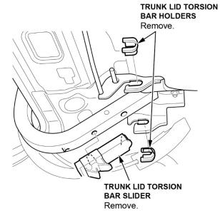
5. Remove the clip and rotate it **180 degrees**.
