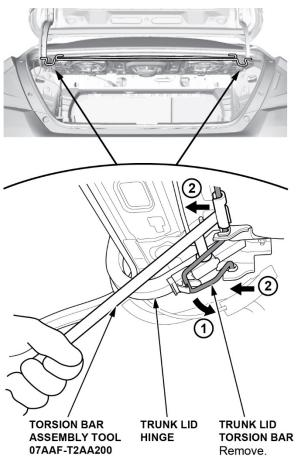
4. If necessary, remove the trunk lid torsion bar holders and the trunk lid torsion bar slider.
