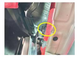
**STEP 6:** While applying slight pressure to the horn to ensure there is no clearance between the horn bracket and the vehicle body, Tighten the horn mounting bolt approximately one full turn.
