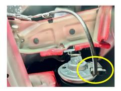
**STEP 5:** Loosen the horn mounting bolt approximately one full turn.
