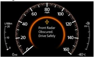
This is caused by inappropriate decision logic of the control software in the front radar sensor. To eliminate this concern, the control software of the front radar sensor has been modified.
