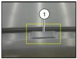
e. Apply adhesive around each clip (1) (on the yellow rectangular areas) after installing "Clip A's" on the vehicle.
