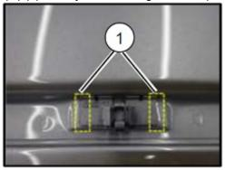
f. Reinstall the roof molding according to the procedure on MGSS (ROOF MOLDING INSTALLATION). 3. Verify the reapir.
