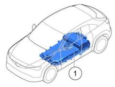
The lead-acid battery is charged by the high-voltage battery when the EV system is activated. If the power is turned ON many times without activating the EV system, the lead-acid battery may discharge completely, making it impossible to turn the ignition ON and to activate the EV system.
