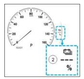
NOTE: When the high voltage battery charge display shows "---", the charge level is 0% or less. If "READY ON" operation is done several times in this situation, the high voltage battery may not keep in a good condition and, in the worst case, it will need to be replaced.
