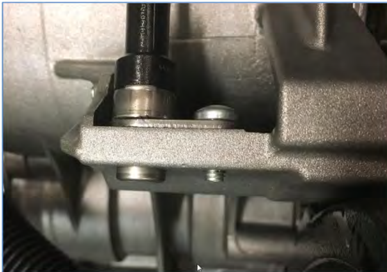
AMT-C/D countershaft speed sensor mounting.
