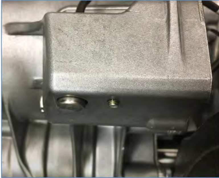
AMT-F countershaft speed sensor mounting.
