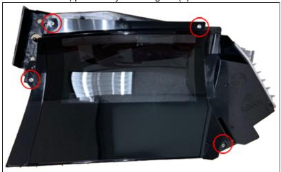
5. Remove the reflective glass bracket by removing one screw as shown.
