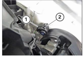
If part number 64 11 5 A3F 255 or 64 11 5 A3F 250 is installed, this must be replaced by a new automatic air recirculation control sensor. Follow ISTA Repair Instruction REP 64 11 991 "Removing and installing sensor for automatic recirculation air control"
