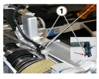
Carefully pinch the tabs on the old vent line and pry it out of the housing (1).
