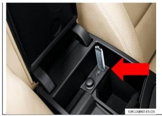
There may be more than one USB connection within the vehicle where the stick can be inserted (center console (arrow), glovebox). However, some vehicles may only recognize the map in one of the USB ports, so try both connections.
