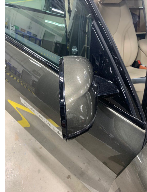
Mirror not being in detent:
