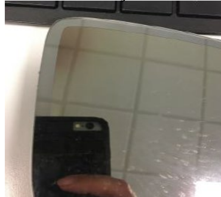
Discoloration of the mirror glass:
