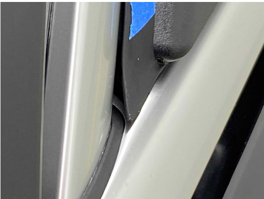
Inconsistent fit of seal to window frame finisher:
