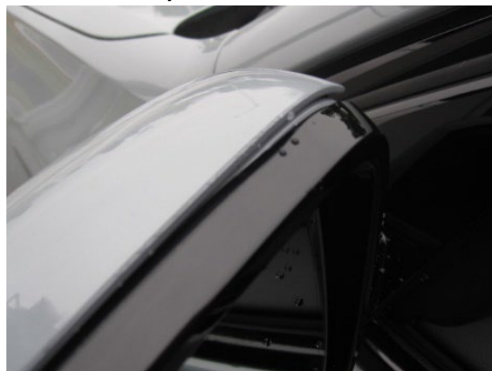
Improper installation of the mirror cap:
