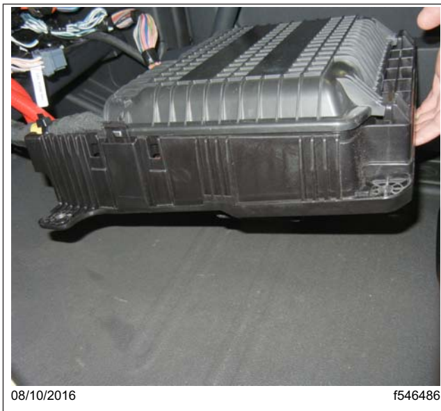
Fig. 15, Lowering the VPDM to the Cab Floor
