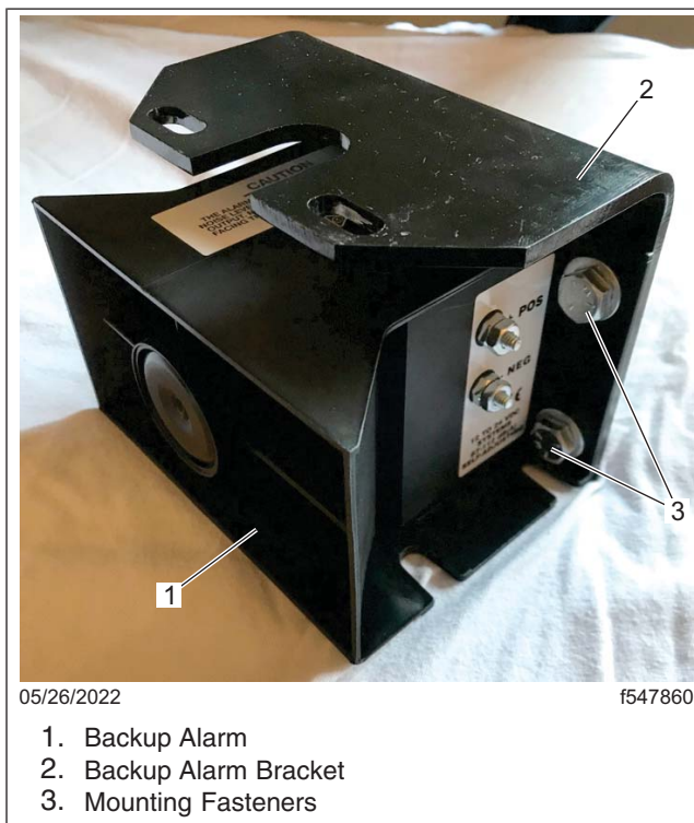
Fig. 10, Mounting the Backup Alarm to the Backup Alarm Bracket
