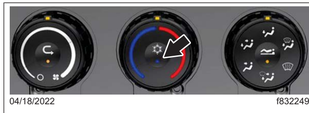
Fig. 1, AC Compressor LED Display
