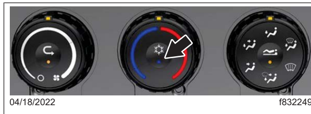
Fig. 1, AC Compressor LED Display
