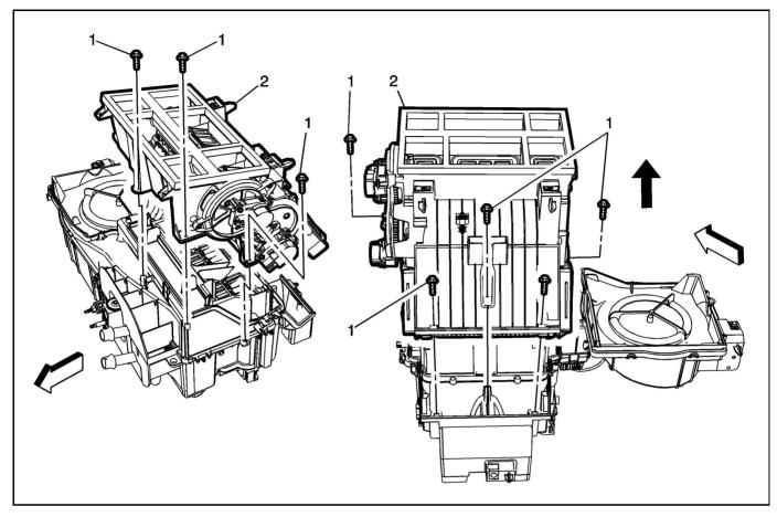
Refer to Air Conditioning (A/C) Evaporator Case Assembly Replacement in SI.
