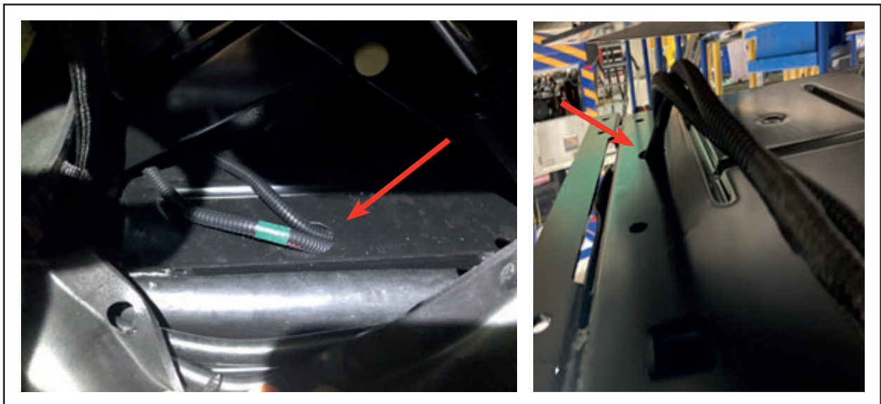
Figure 5 - Secure the harness in Bottom of Baseplate
