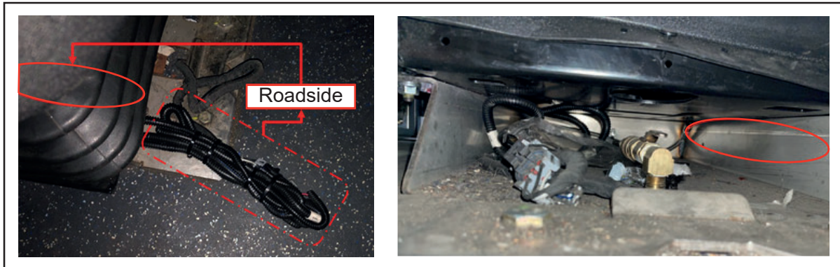
Figure 4 - Secure the harness under the Driver Seat Frame
