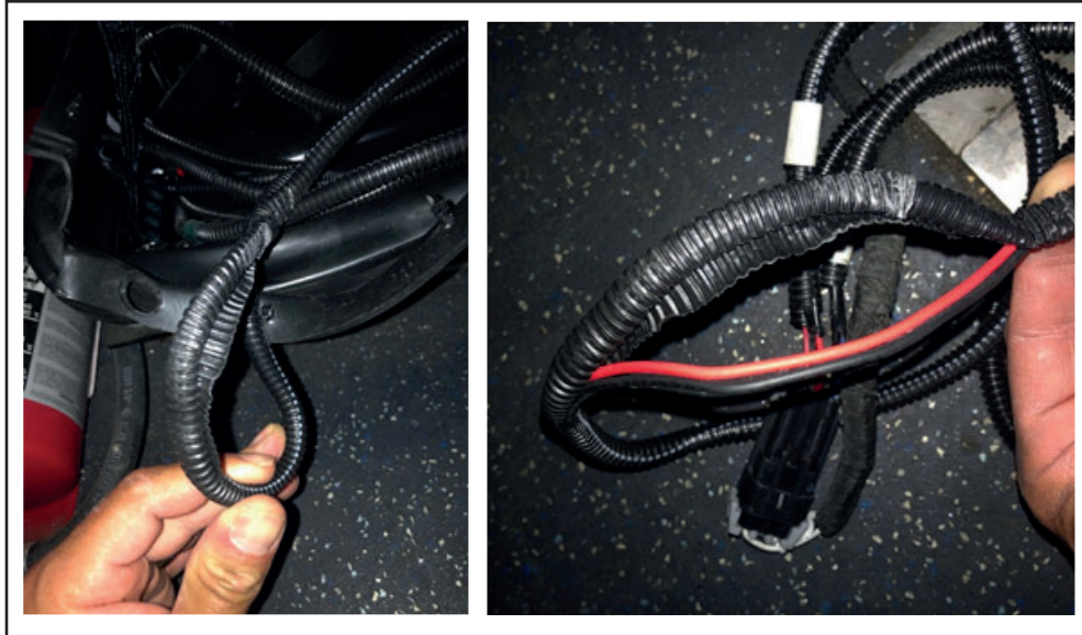
Figure 2 - Inspection of damaged Seat Belt Harness
