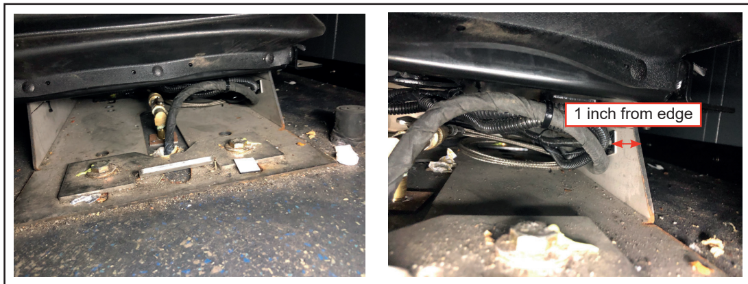
Figure 7 - Secure the SeatBelt harness to Tie Mounts
