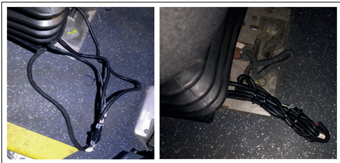
Figure 3 - Secure the Harness with Zip ties
