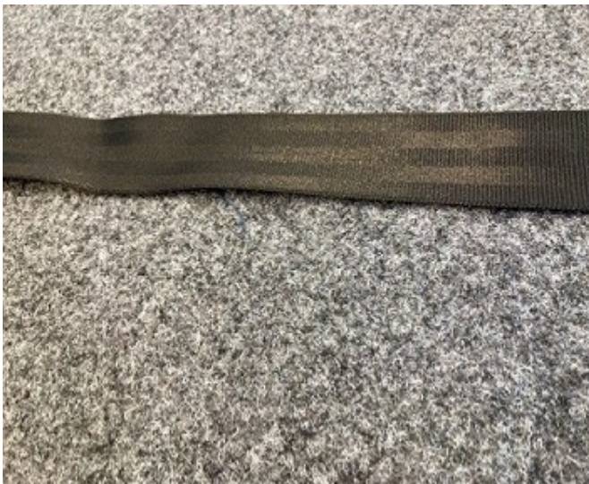
Figure 2. Waviness indicates that the seat belt was pulled on when exiting the rear of the vehicle
