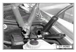
When using remote location terminals -arrows-, located in engine compartment, always reduce DIN rating on VAS6161 and GRX3000VAS testers.
