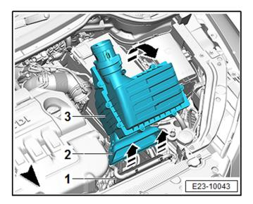
• Pivot the air filter housing <3> rearward in the direction of <arrow>. At the same time remove the air duct <2> from the air duct <1>.
