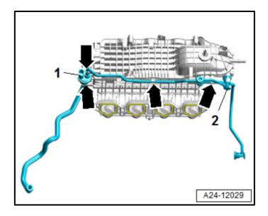
Replace EVAP Canister Purge Regulator Valve 1 -N80- with connecting pipe.
