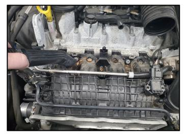
Vacuum any debris that has accumulated on top of the intake manifold
