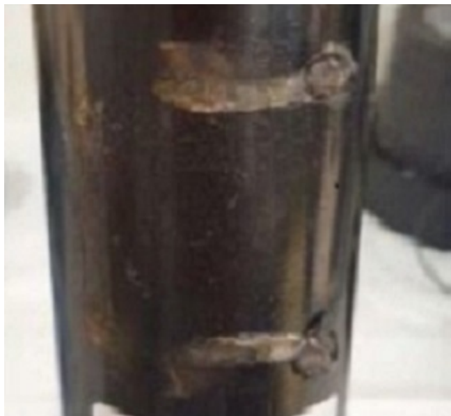
Fig. 2 Strut With Sway Bar Ear Broken
