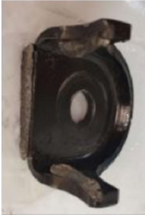
Fig. 1 Sway Bar Ear Broken
