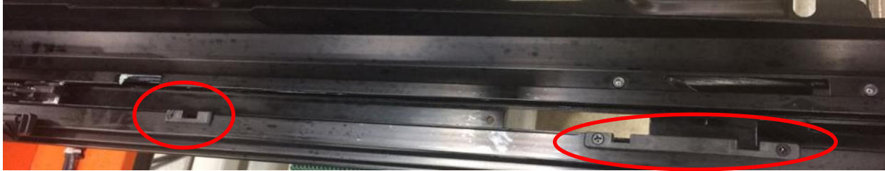
Fig1. Apply white lithium lubricant to the areas shown on frame. 1 side shown- apply to both sides.
