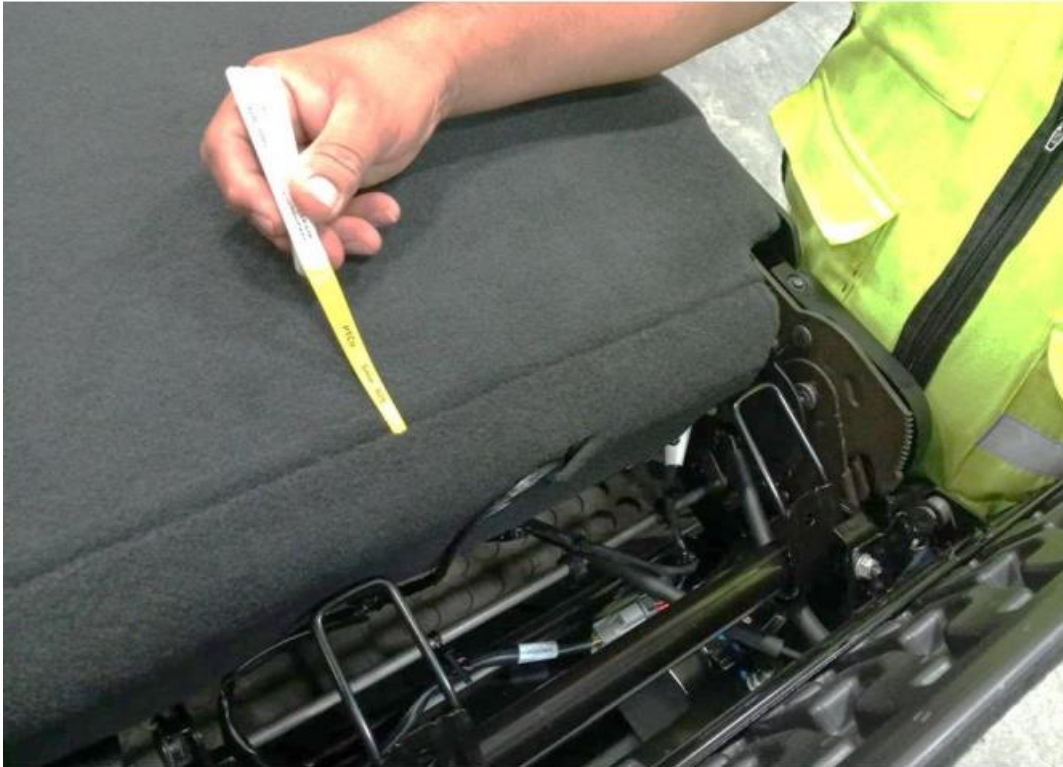
Fig 2 Trim stick used to seat the J channel retainer.
