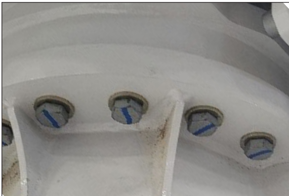
Figure 1 — Outer Race Rotation Bearing Cap Screws and Washers
