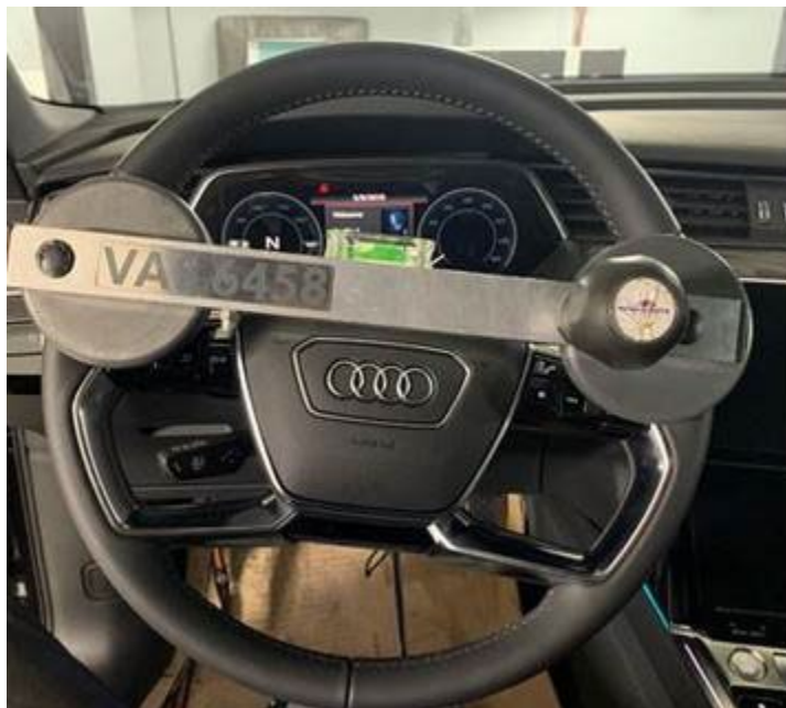
Figure 1. VAS 6458 installed with steering wheel off-center.
