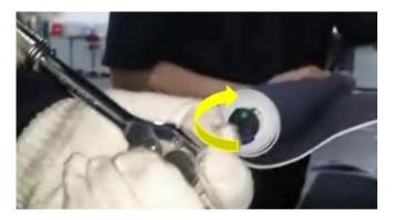
With the aid of a second person, hold the sunshade material tight against the reel so that it cannot unwind. Insert a 6 mm hex socket into the end of the sunshade. Remove the locking pin. DO NOT ALLOW THE SHADE TO UNWIND.
