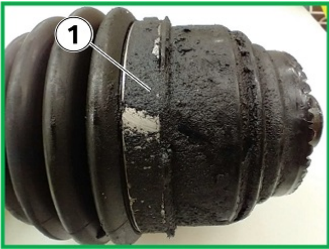
Example of dirt/contamination from outside influence (1).
