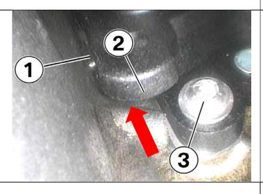
Continue to push bore scope downward towards the plastic vacuum reservoir tab (2).
