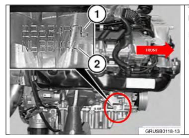
The engine serial number is located at the lower front right corner of the engine block.
