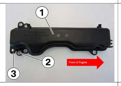
It is possible that a black plastic vacuum reservoir (1) is installed. This illustration provides an overview of the entire component and specific points of the component.
