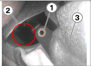
After inserting the bore scope, you must locate the cylinder head gasket tab. (1).
