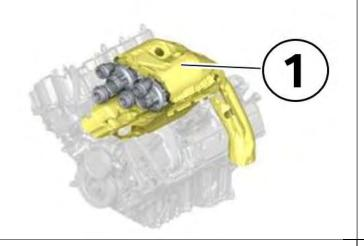
Remove the heat shield (1) to diagnose the engine oil leak.
