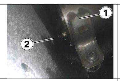
Continue to push the bore scope towards the vacuum reservoir (1). The engine valley drain hole is location is just to the left of the vacuum reservoir (2).
