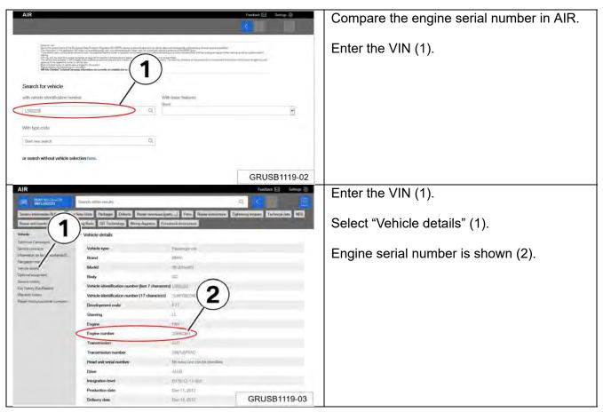
If the serial numbers do not match, then create a TSARA TeileClearing Hotline case with the numbers that are shown on the engine block and wait for a response before proceeding with repairs.
