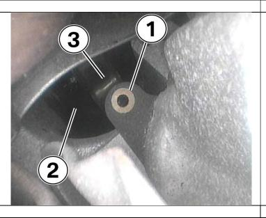
Feed the bore scope past the left side (1) of the cylinder head gasket tab (2) towards the vacuum reservoir (3).
