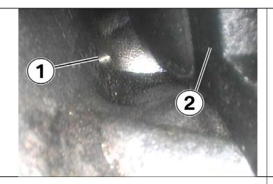
Once the bore scope has gone under the plastic reservoir tab then the engine valley drain hole (1) and surrounding area can be clearly inspected.
