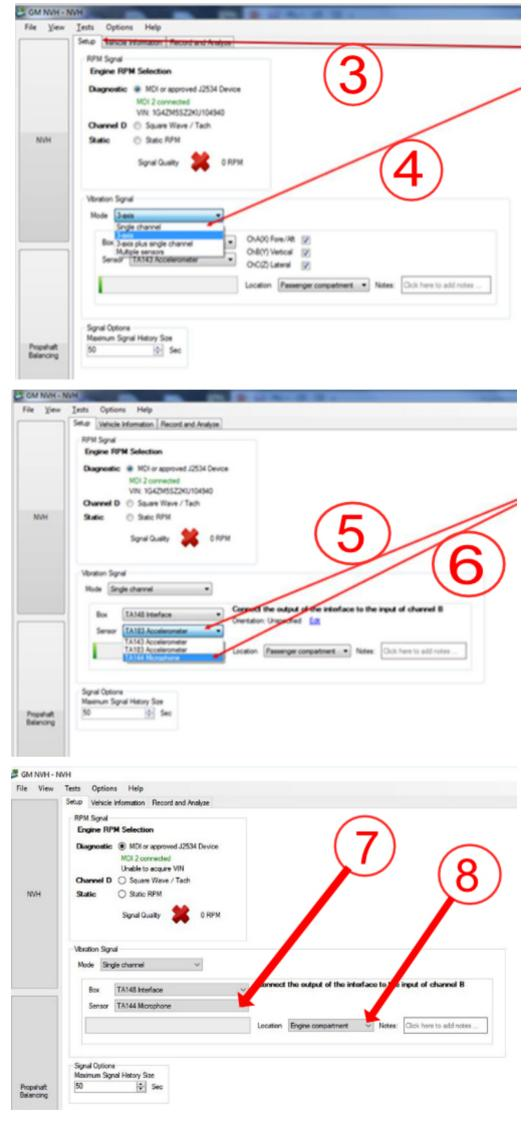
Note: If using 3 axis, use center channel only and set up as single axis.
