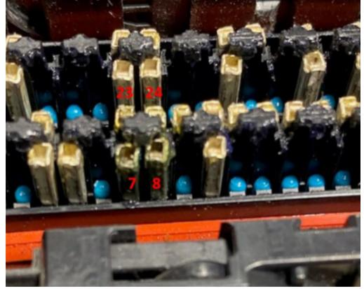
3. If coolant corrosion or discoloration is found, replace circuits 410 and 2761 from the engine coolant temperature sensor (ECT) to ECM connector X3. Replace the coolant temperature sensor and replace or clean connector X3 at the ECM.
