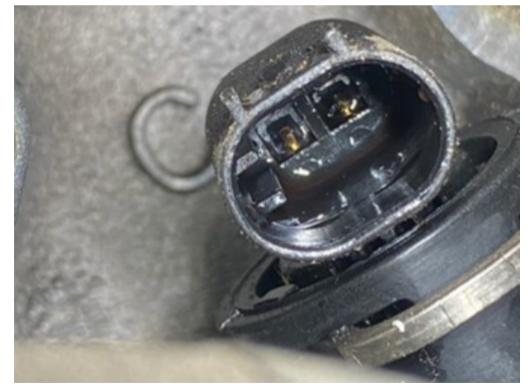
2. Trace the circuits back to the X3 connector at the ECM and inspect for coolant contamination / corrosion.
