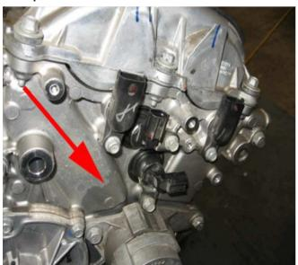
The engine illustrated above shows residual oil staining from assembly. There are no drips or leak paths present.
