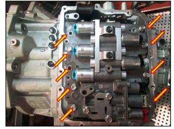
17. Reinstall the bolt that secures the detent spring and tighten the bolt to specification.
