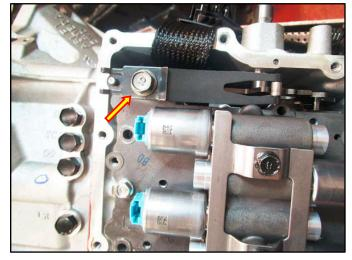
18. Reconnect the solenoid harness to the solenoids and install the oil temperature sensor.
