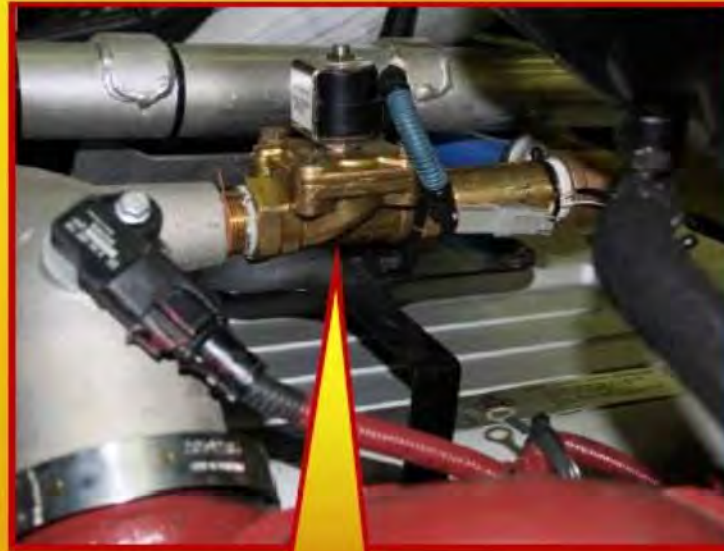
DPF Combustion Air Valve
