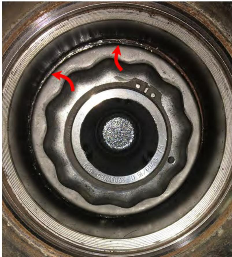
Presence of grease around the o-ring indicates a leaking bearing
