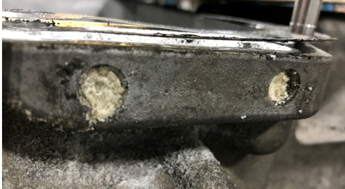
Clogged vent ports
