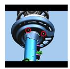
3. Visually inspect the lower spring isolators to ensure that they are properly oriented/aligned in the spring isolator, as shown in the picture above.
