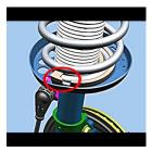
2. Visually inspect the spring orientation to the lower isolator is nested to the stopper in the lower isolator, as shown in the picture above.
