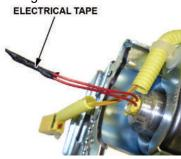
3.3. Tape the twisted ends with electrical tape.
