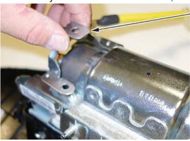
INFLATOR BRACKET Do not reuse. 5. Remove the inflator by pulling it out.
