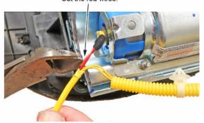
3.2. Strip away about **1 inch** of the red wire insulation, then twist the wires together.
