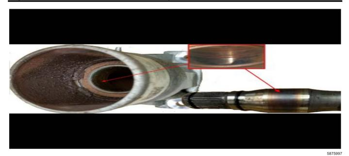
**Note:** Fretting worn IDS Shaft and Bracket must discarded and replaced with new parts. Replace the housing only if damage has been verified.
