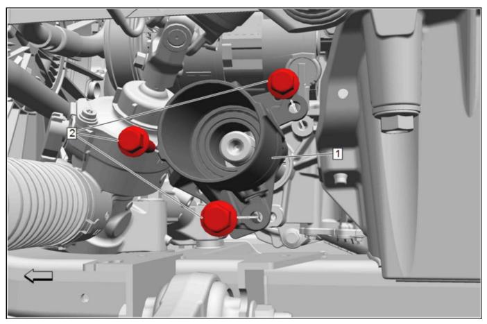
Remove the Front Wheel Drive Intermediate Shaft Housing (1). Refer to Front Wheel Drive Intermediate Shaft Housing Replacement in SI.
