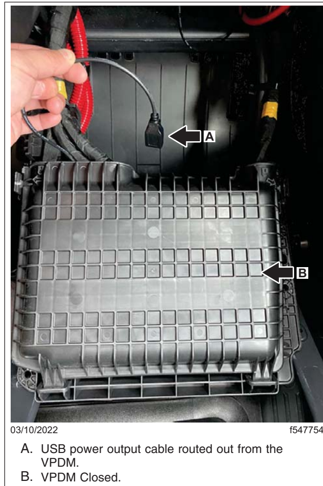
Fig. 21, USB Power Output Cable Routed Out from the VPDM
