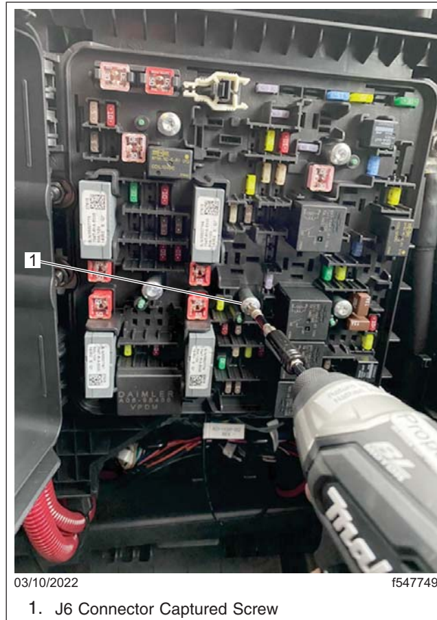
Fig. 14, J6 Connector Captured Screw
