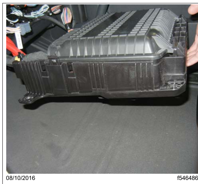
Fig. 15, Lowering the VPDM to the Cab Floor
