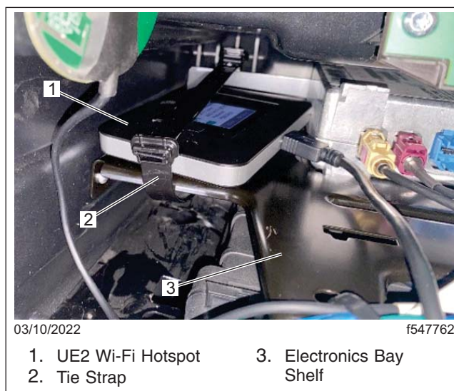
Fig. 41, UE2 Wi-Fi Hotspot Device Installed
