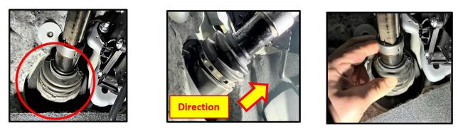
**STEP 2:** Push the dust seal in a downward direction away from the steering wheel. This will allow the old grease to be exposed.
