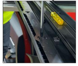
4. Add noise reduction material from the Interior Noise Kit (see below) anywhere the trim makes contact with the frame.
