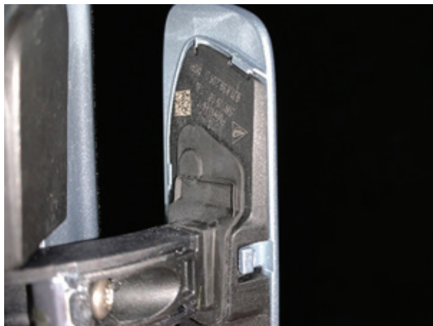
Figure 3: Manufacturing Stamp on Door Handle
