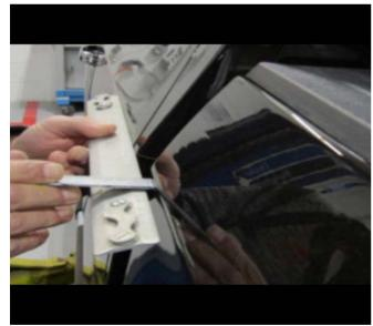
**Note:** Measure the cab to box distance on both sides of the vehicle.
