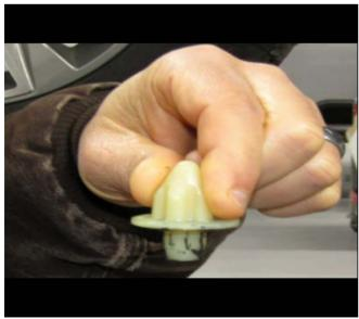
**Note:** If box alignment is limited due to locating pins in the bed preventing correct alignment, the front locating pin can be removed.
