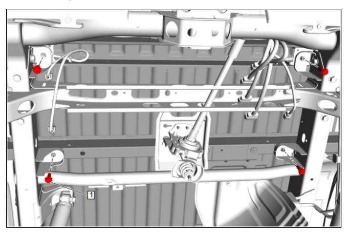
3. Remove the 4 **rear** pickup box bolts (1) and clean any sealer that may prevent movement between the bolt and frame. Reinstall the bolts and hand turn a couple of turns.
