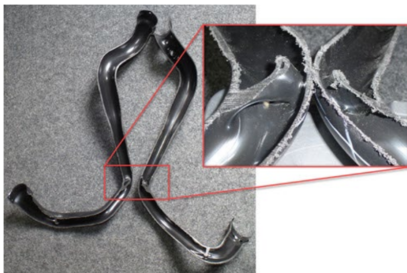
Figure 1. Material accumulation in the charge air pipe.
