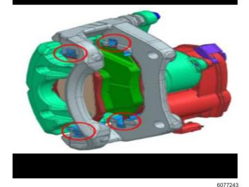
Note: There are 4 Pad abutments per caliper.
