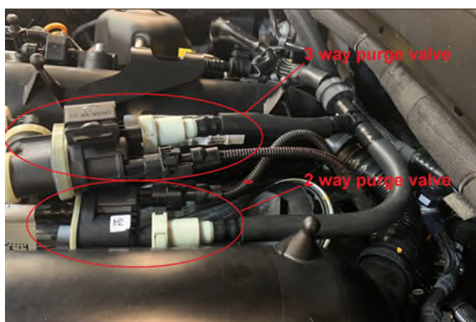
High load purge line on V8 engine.
