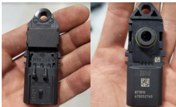
Picture 3 – Blow-by pressure sensor (F160)
