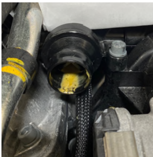
Picture 6 – Blow-by valve contamination check
