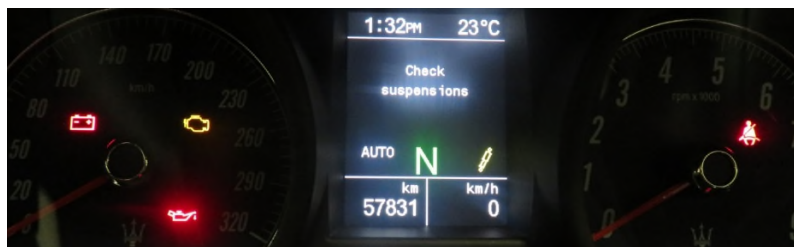
Figure 1: error message on the NQS display and Active Suspensions warning light.
