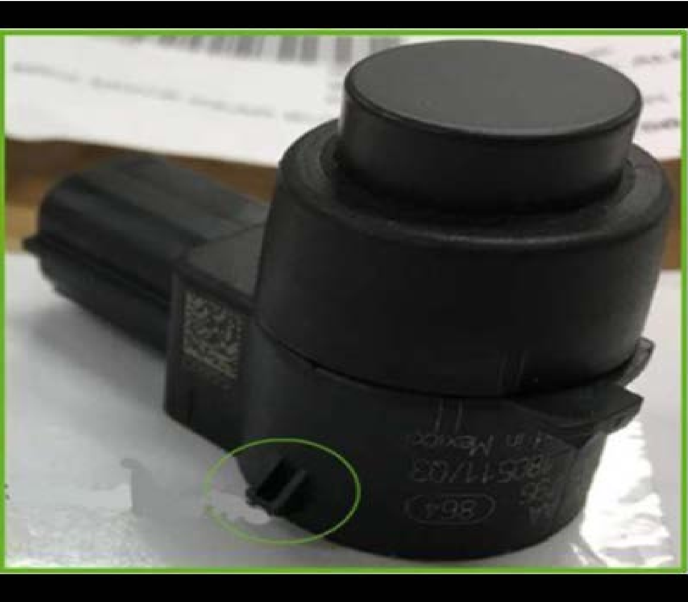
– Good sensor with no retaining tab damage.
