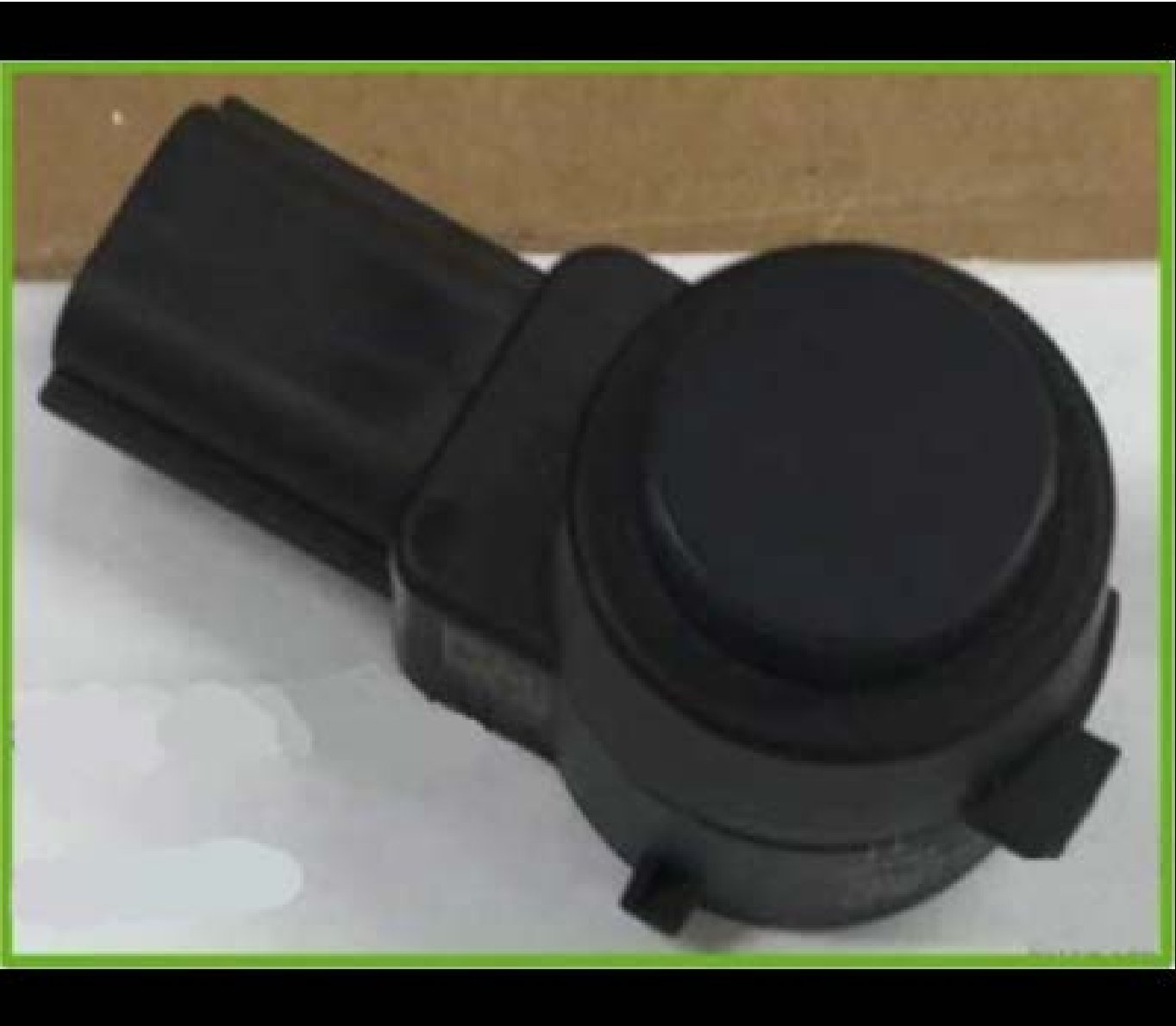
– Good sensor with correct amount of paint.
