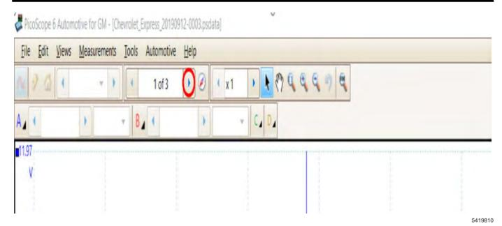
Use the waveform Buffer button to move to the next window.
